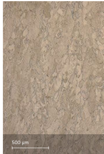
Microstructure solution annealed Etched with etchant Kallings 2
