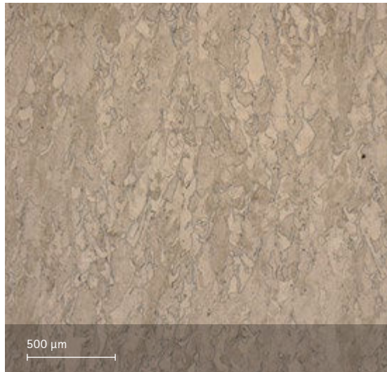
Microstructure solution annealed Etched with etchant Kallings 2
