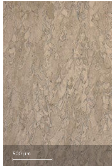
Microstructure solution annealed Etched with etchant Kallings 2
