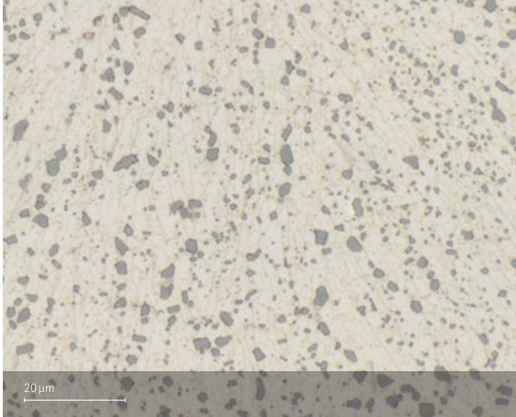
Heat treated microstructure. Etched according to internal procedure using Groesbeck reagent.
